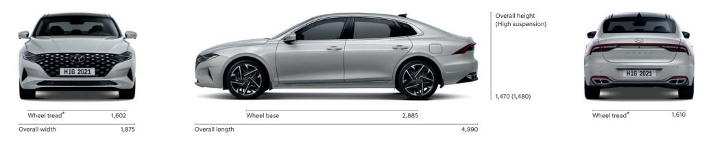
Unit : mm \* Wheel tread • 17" Alloy wheel (Front / Rear) : 1,612 / 1,620 • 18" Alloy wheel (Front / Rear) : 1,607 / 1,615 • 19" Alloy wheel (Front / Rear) : 1,602 / 1,610
