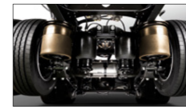
Rear Air Suspension The rear air cushion maintains a stable vehicle posture for better ride comfort while also allowing the adjustment of the cargo bed height when loading and unloading.
