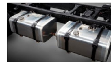
200L+200L Dual aluminum fuel tanks
