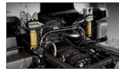
Cab Air Suspension It mitigates cab vibrations and shocks and minimizes cab roll during turning maneuvers to provide a comfortable, stable and quiet ride.
