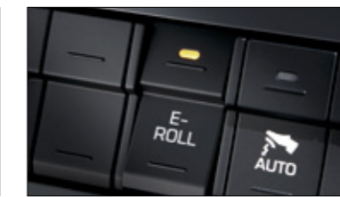
Advanced Eco Roll Shifts into neutral gear improve fuel efficiency to improve fuel economy by 2-3% by taking advantage of downhill coasting and flat runs. (Apply on M/T)
